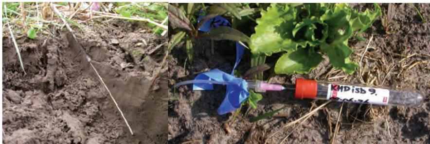
Figure 5. Lysimeter installed in the field for sampling soil solution (Papers I, II). Soil has been excavated to show the position of the lysimeter. Photo: Ines Barth and Kerstin Huss-Danell.
